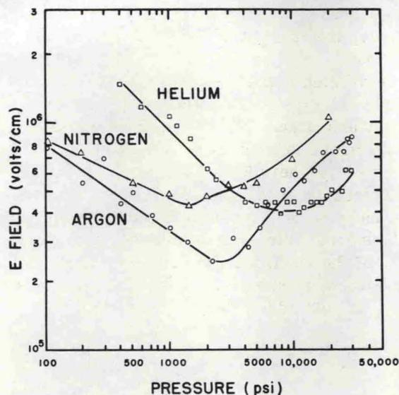
FIG. 2. Pressure dependence of breakdown field strength.
